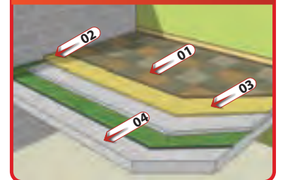
DETAIL OF CARPETED FLOOR WITH PRODEX ® UNDERCARPET
