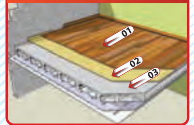
DETAIL OF A PRE-TENSIONED COMPOSITE FLOOR WITH PRODEX ® UNDERFLOOR
